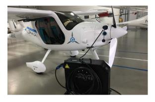
The general aviation/recreational aircraft group consists of aircraft with MTOW from 300 to 1000 kg. These are mostly electric powered aircraft with a seat capacity of two. This category includes aircraft which are already produced and certified, for example the Pipistrel Alpha Electro.
