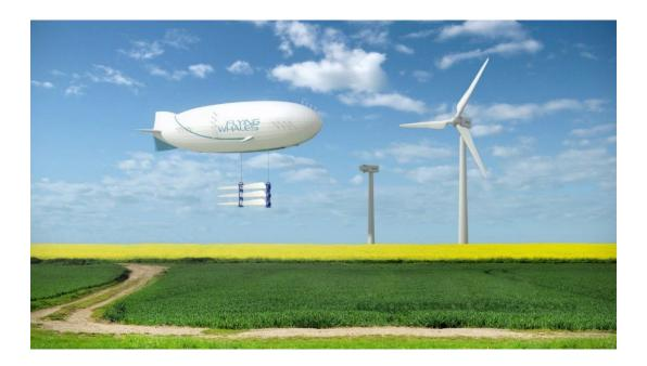
Pushing the limits further, a 100% LTA aircraft relies only on buoyancy to stay airborne. This aerostatic, as opposed to aerodynamic, lift means that the LTA needs no energy to fly. Its propulsion system will be dedicated to cruise – as it has no need to fight gravity – while airborne and maintains a stationary position during hovering, to load and unload cargo. In this perspective, an LTA aircraft can save up to 98% of carbon emissions depending on the type of mission.<sup>9</sup>
