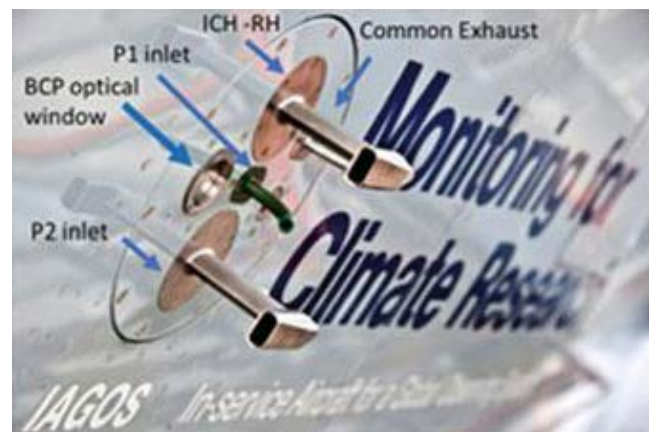
FIGURE 1: The inlet plate used on IAGOS-CORE aircraft.
