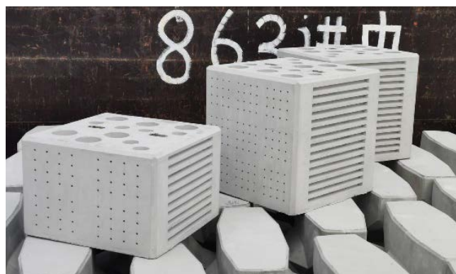
FIGURE 3: Eco-enhanced blocks to be deployed on sloping seawall.
