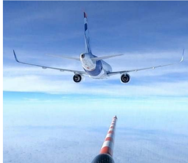
FIGURE 3: Foto taken from the cockpit of the DLR research aircraft Falcon chasing an Airbus A320neo in 50 m distance to probe the emissions from its CFM LEAP-1A engines during the NEOFUELS/VOLCAN project coordinated by Airbus and DLR (Voigt et al., 2025 submitted; https://www.dlr.de/de/medien/videos/2023/video-projekt-volcan )
