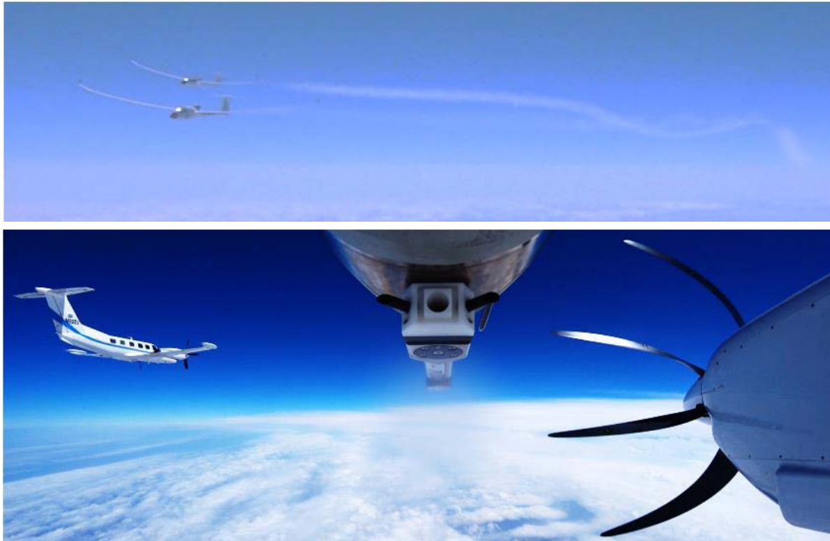
FIGURE 2: (upper panel) Picture of the Blue Condor glider equipped with a hydrogen engine (front) and a kerosene engine (back) both forming contrails of different optical thickness (Rogero et al., 2024; https://www.dlr.de/en/latest/news/2025/world-first-in-flight-measurements-of-contrails-from-hydrogen-propulsion ). (lower panel) Picture taken from the instrumented chase aircraft Egrett during contrail and emission measurement of a turbo prop aircraft equipped with a water release system simulating fuel cell emissions (Neumann et al., 2025).
