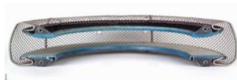
*Figure:* engine intake treated lips
