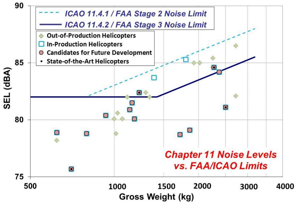
Figure A-4. Chapter 11 Certification Noise Levels vs. 11.4.1 and 11.4.2 Noise Limits
