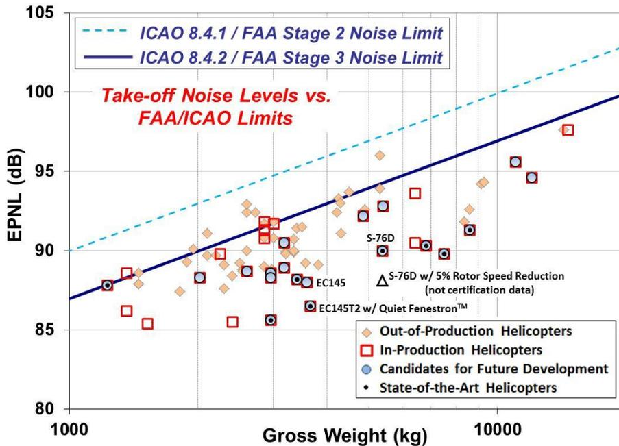
Figure 6. Chapter 8 Take-off Noise Levels vs. Gross Weight Showing Current Best-in-Fleet Margin to 8.4.1 and 8.4.2 Limits and Example Case of  $N_R$  Reduction
