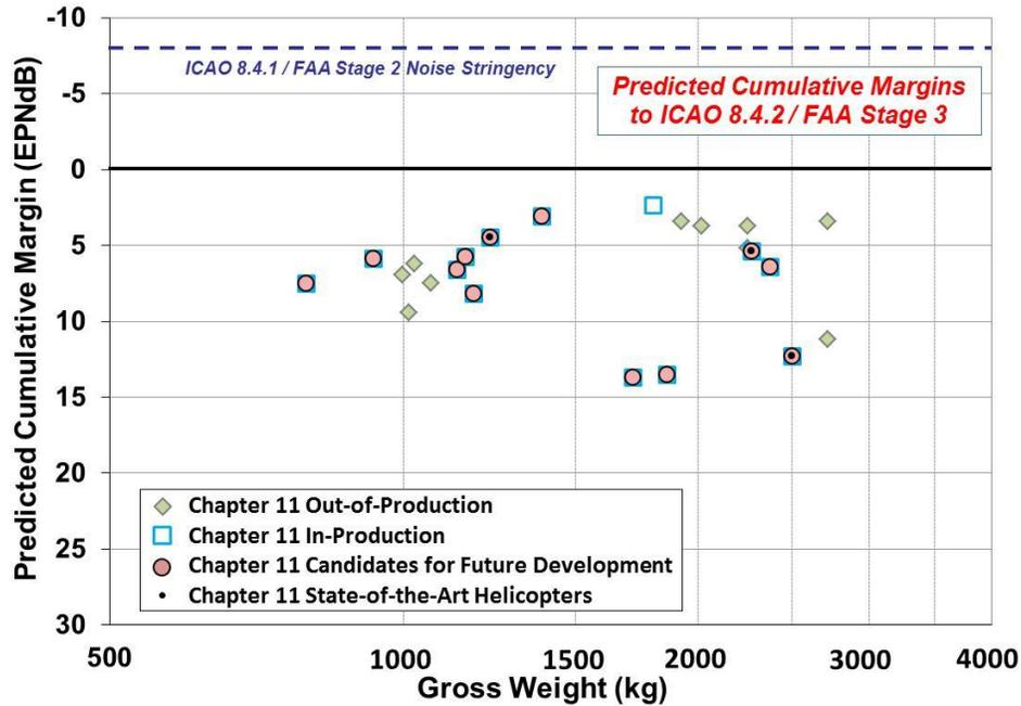
**Figure 2. Predicted Cumulative Margins to 8.4.2 Noise Limits for Chapter 11 Helicopters**
