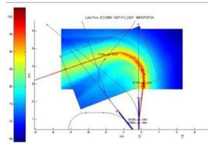
*Figure:* Noise footprint prediction of a turn, flown by an EC130
