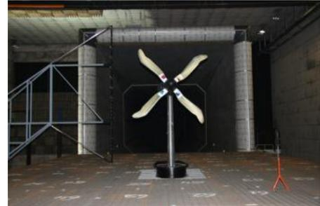
*Figure:* ADYN rotor in DNW-LLF wind tunnel
