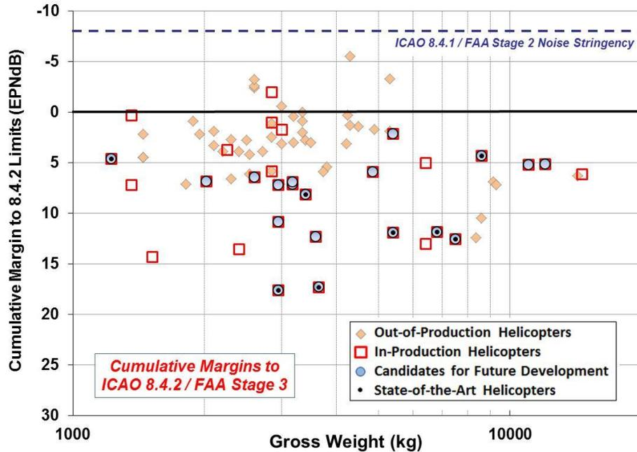
**Figure 1. Cumulative Margins to 8.4.2 Noise Limits for Chapter 8 Helicopters**
