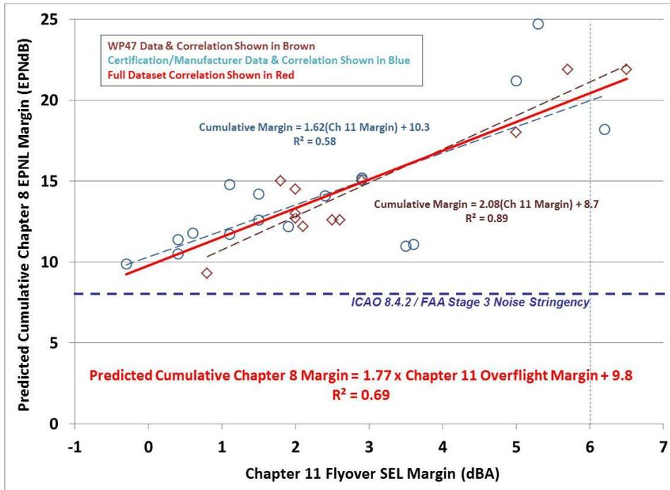
**Figure B-1. Correlation of Cumulative Margins to Chapter 8 Noise Limits vs. Margins to Chapter 11 Overflight Noise Limit (Cumulative 8.4.1/Stage 2 Margins vs. 11.4.1/Stage 2 Overflight Noise Margins)**
