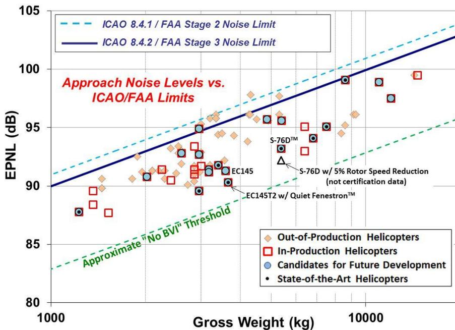
Figure 7. Chapter 8 Approach Noise Levels vs. Gross Weight Showing Current Best-in-Fleet Margin to 8.4.1 and 8.4.2 Limits, Example Case of  $N_R$  Reduction, and Approximate “No BVI” Margin Threshold
