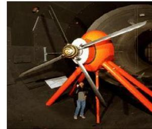
*Figure:* active flap rotor in S1-Modane wind tunnel
