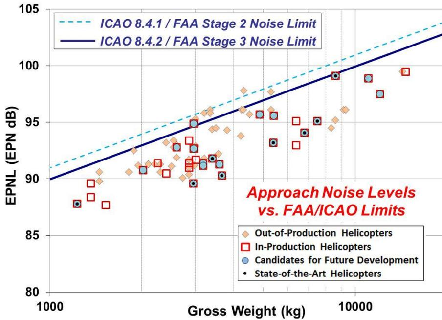
Figure A-2. Chapter 8 Approach Certification Noise Levels vs. 8.4.1 and 8.4.2 Noise Limits
