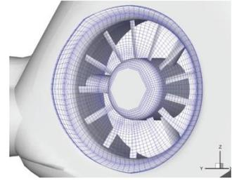
*Figure:* Fenestron noise computation – Acoustic integration surfaces
