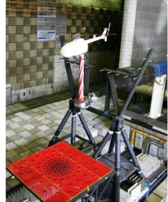
*Figure:* HELINOVI-Model in DNW-LLF wind tunnel
