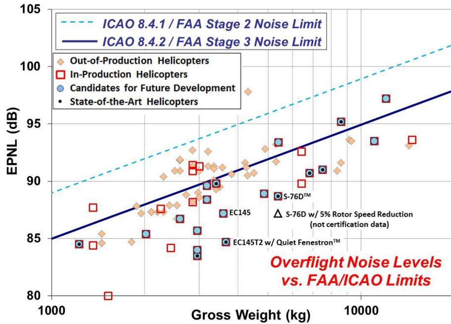
Figure 8. Chapter 8 Overflight Noise Levels vs. Gross Weight Showing Current Best-in-Fleet Margin to 8.4.1 and 8.4.2 Limits and Example Case of  $N_R$  Reduction
