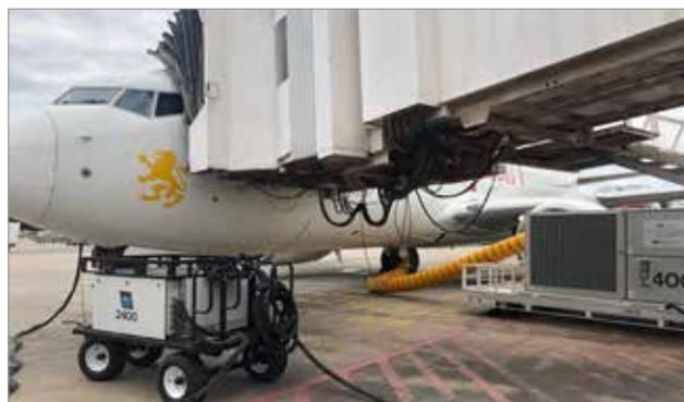
Gate equipment (GPU and PCA) funded by the project is connected for the first time to an international flight at Moi International Airport, Mombasa, Kenya
