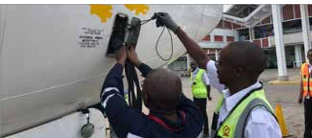
Gate equipment (GPU) is being connected to power aircraft during ground operations which avoids the use of jet-fuel powered APUs
