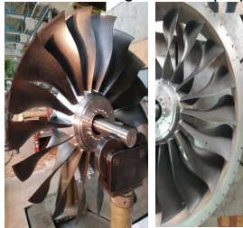
Rotor of the fan model C194-2 with composite blades
