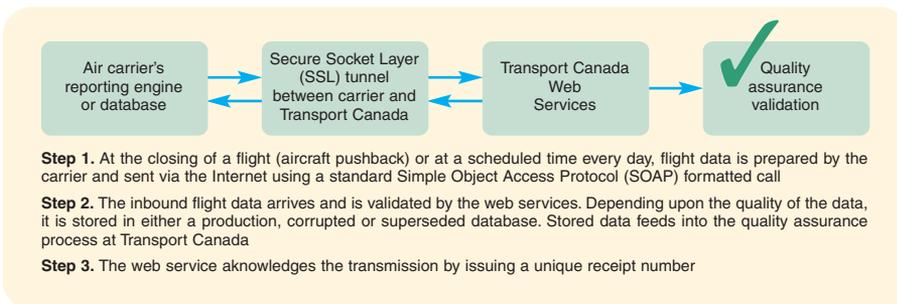
**Structure of an ECATS web service call: the bidirectional transmission is completed once the carrier receives a response, a process that requires about three seconds**
