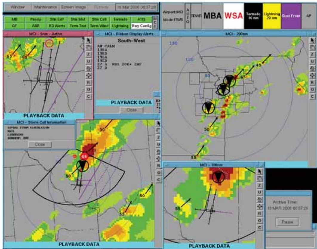
Example of ITWS display of severe weather containing microbursts, a gust front and tornados (Kansas City, 13 March 2006). ITWS features a prediction product that forewarns of a microburst
