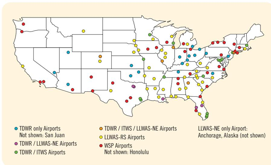
**Location of FAA terminal wind shear and weather systems. In addition to sites shown, four LLWAS-NE systems are collocated with TDWR, and five LLWAS-NE systems are collocated with TDWR and ITWS. As of 2 February 2007, 13 ITWSs serve 23 aerodromes equipped with TDWRs**
