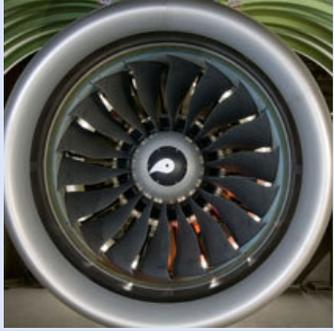
**Pratt & Whitney's** geared turbofan engine (**PW1000G engine**) to be used in Bombardier Inc.'s C Series and the Mitsubishi Regional Jet - is said to **reduce fuel burn by 12 per cent** compared to the company's most efficient engine on the market.
