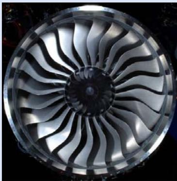
**Rolls-Royce BR725** - Compared with the highly successful BR710, the BR725 is more powerful, has **4 per cent better specific fuel consumption and shows a 21 per cent improvement in NOx emissions**. Design features include a 50-inch diameter fan assembly made up of 24 “swept” titanium blades for improved aerodynamic efficiency and lower noise. Flight test engines being delivered to Gulfstream towards the end of 2008.
