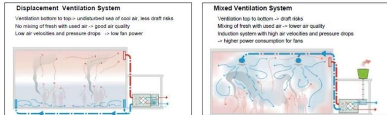
By displacement ventilation system, the air is supplied near the floor to a distance of 10-15m and exhausted near the ceiling. This requires lower air volume movement rates, leading to lower fresh air intake rates and less electricity required to drive the fan for both air exhaust and supply.
