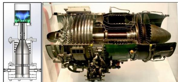
*Left: Experimental setup CAD design and superimposed notional flame image. Right: typical J85 engine available for test.*
