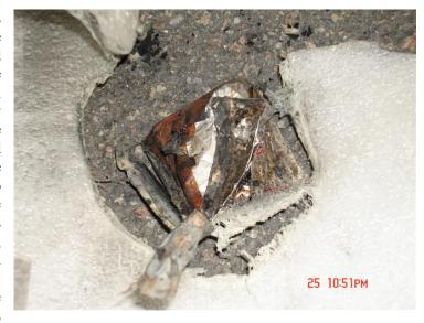
hazardous. The inner contents were discovered to be 33 GPS trackers bundled together in groups of five. Each device was sealed in clear plastic and each GPS consisted of a circuit board, battery and a tubular type container with a red top. It appears that two of the devices heated, causing the surrounding packaging and cushioning to ignite. The surrounding foam wrap melted.
