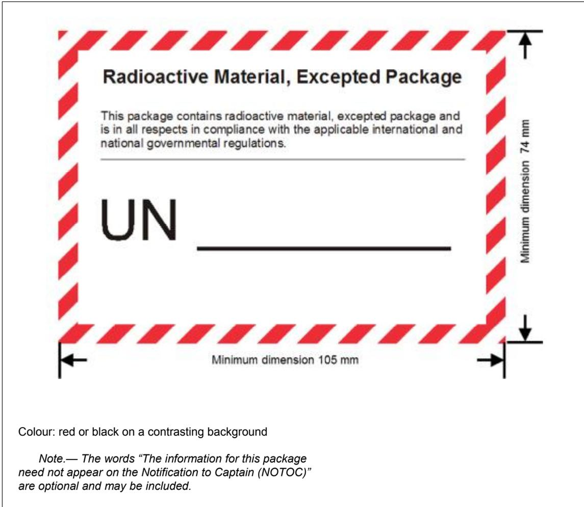
**Figure 5-31. Radioactive material, excepted package**
