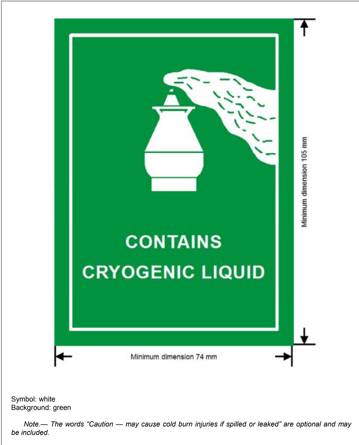
Figure 5-29. Cryogenic liquid label
