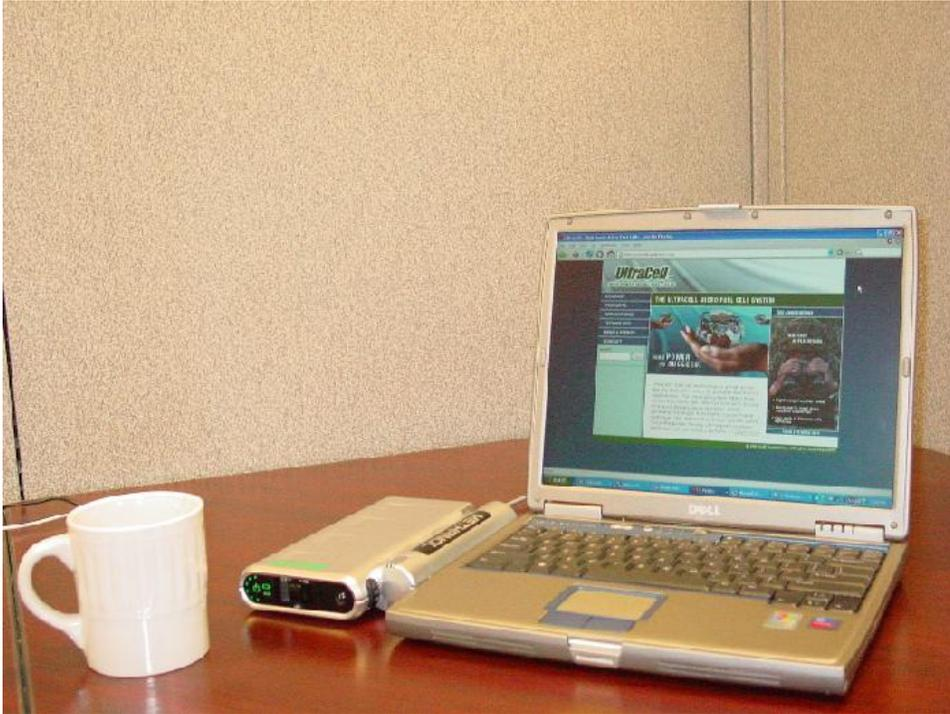
**Figure 7.** An UltraCell RMFC system for laptop computers
