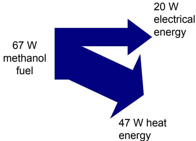
**Figure 4.** Energy flows for a 20 W RMFC and DMFC systems running at equivalent net efficiencies
