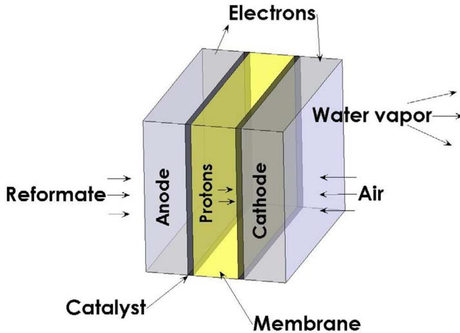
**Figure 1.** Diagram of a single cell
