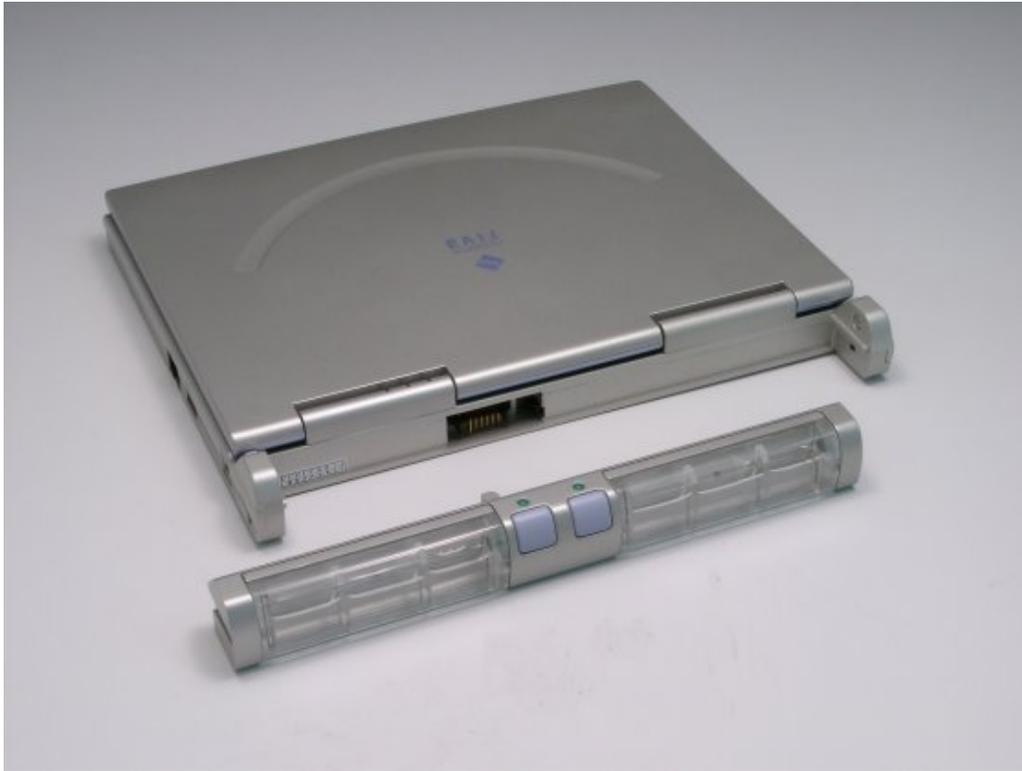
**Figure 8.** Image model of a Casio RMFC system for laptop computers
