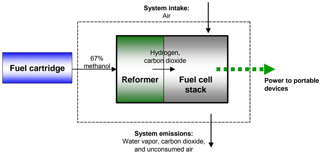
**Figure1.** Basic schematic of a micro RMFC\*
