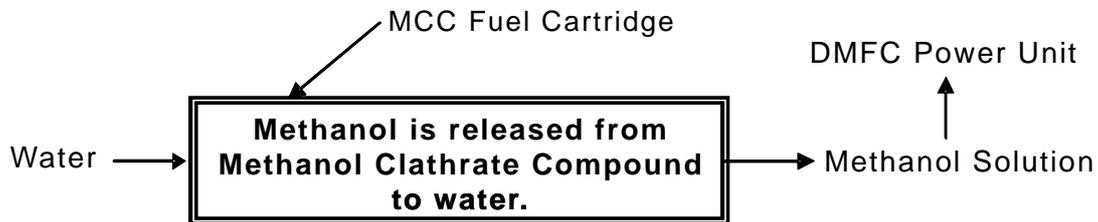
**Figure 3** Usage of MCC with DMFC power unit
