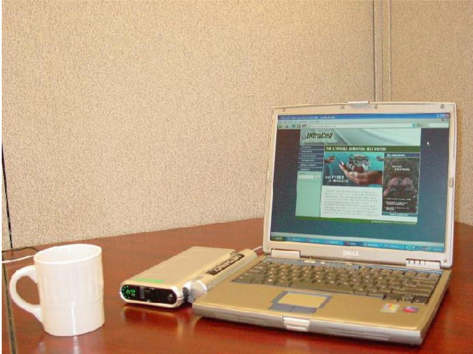
**Figure 6.** An UltraCell RMFC system for laptop computers
