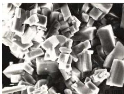
**Figure 2** Electron microscope photograph of MCC.
