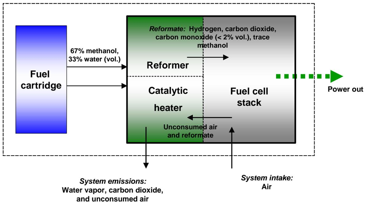
Figure 5. Detail of gas and liquid flows in RMFCs
