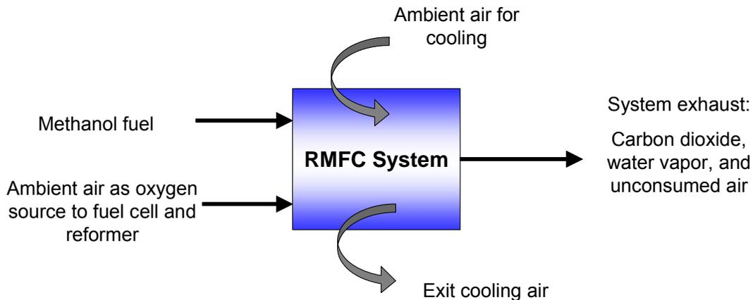
**Figure 2.** Liquid and gas flows in an RMFC
