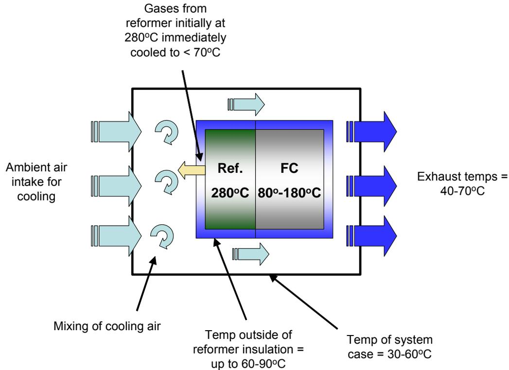
**Figure 3.** Thermal management in a micro RMFC
