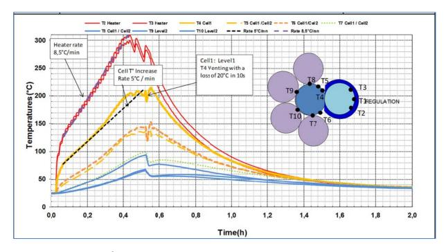
ANNEX 2: <u>Tests on 4<sup>th</sup> segment: large Li-rechargeable cells/batteries for industrial and automotive uses, as well as energy storage in homes</u>
