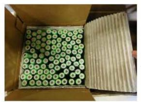
"Thermal Management System" (TMS) by Fireproof Solutions, Inc. Comprised of "cooling inserts" (treated corrugated) to contain thermal runaway
