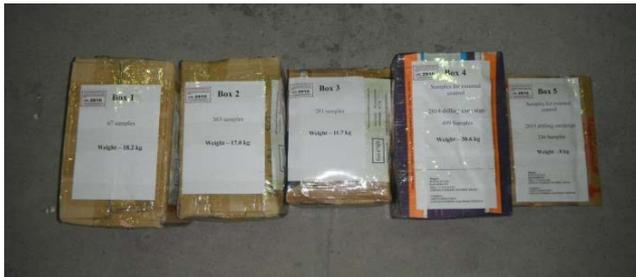
Plastic bags are gathered in fibreboard boxes (from few kg to few tens of kg each), placed in a plywood outer box. The whole package is UN2910
