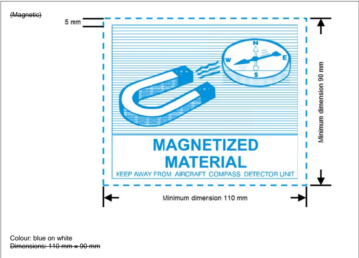
Figure 5-24. Magnetized material
