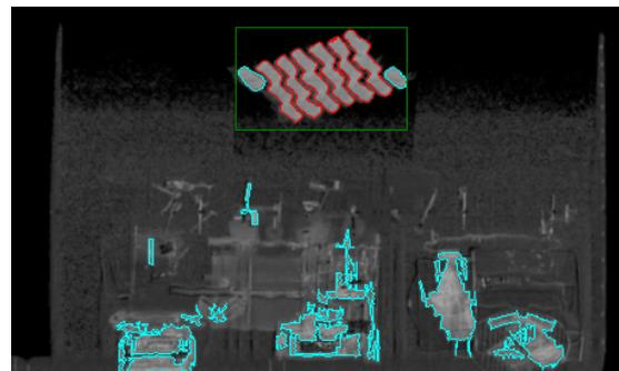
LSH20 D size Li-metal batteries attached to cargo
