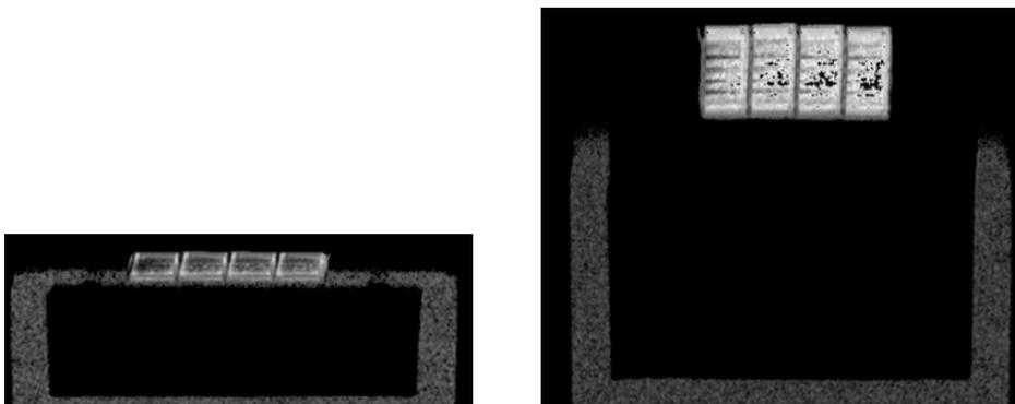
Figure 9. Comparison of two side-view Zeff images of D-size alkaline batteries. In the left image, the batteries appear long and thin and the Zeff image is dimmer (i.e. lower Zeff values) than on the right. The image on the left has a mean Zeff of ~9 while the image on the right has a mean Zeff of ~16, which is closer to the values obtained for the top-view images shown in Figure 25.
