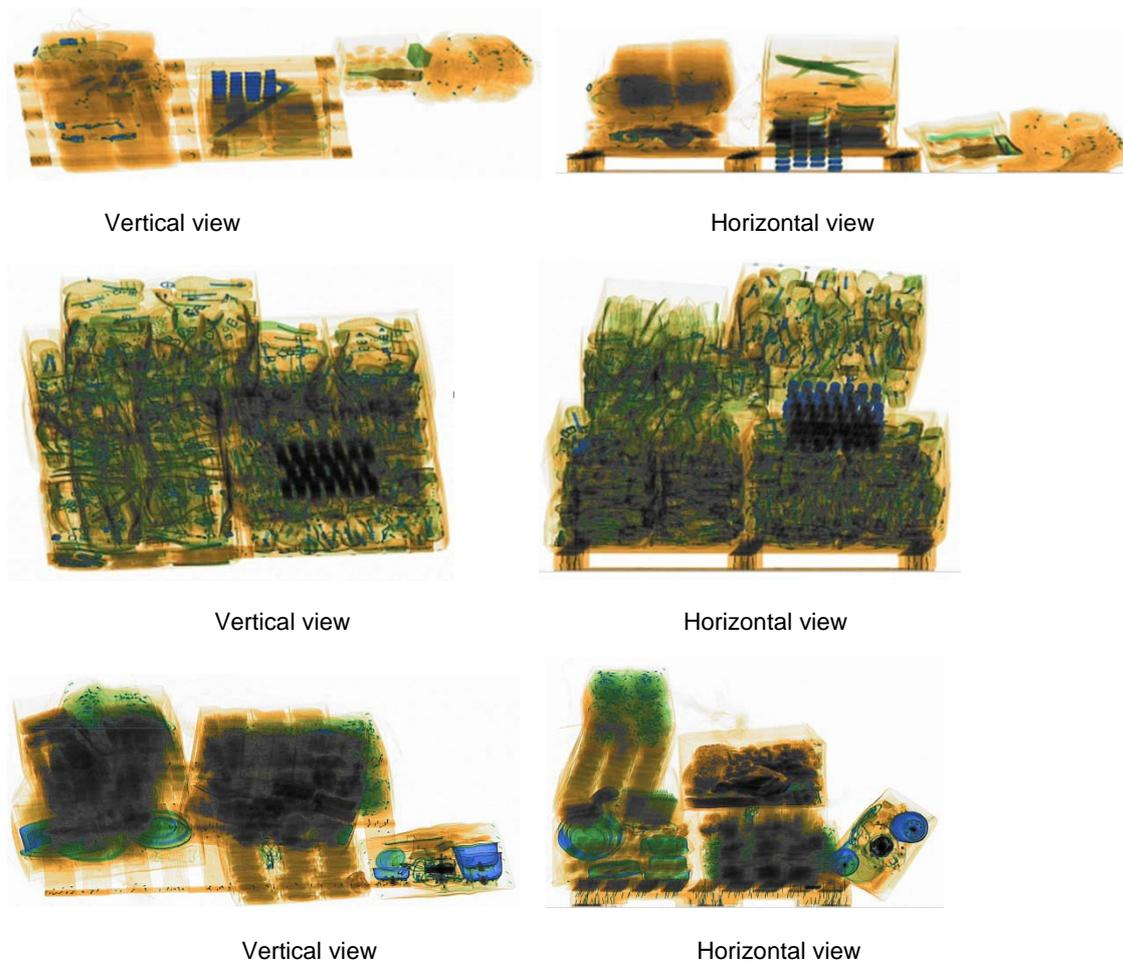
Figure 5. X-ray images of batteries attached to cargo. First row: low clutter. Second row: moderate clutter. Third row: high clutter.
