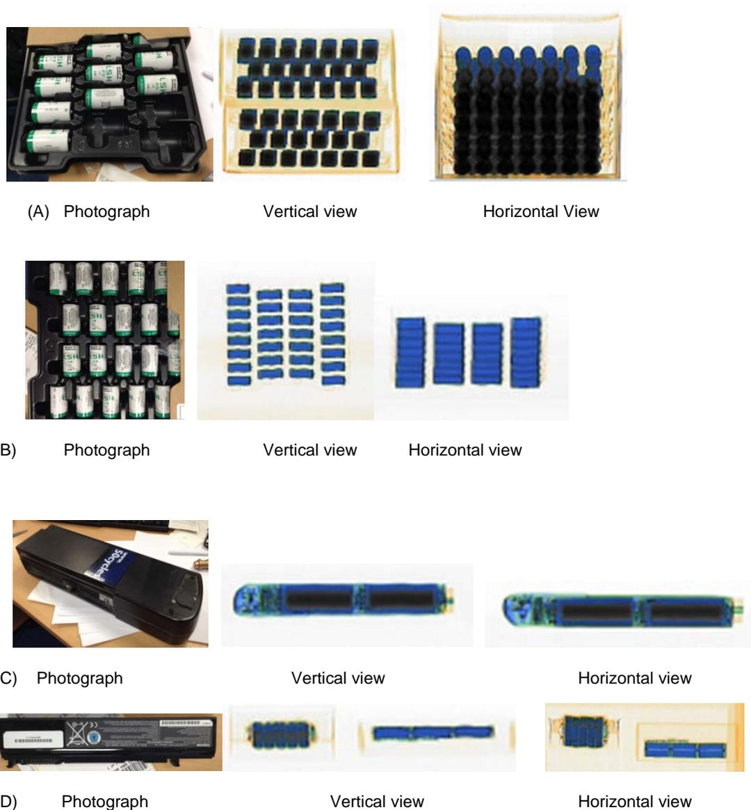
Figure 4. X-ray images of bare batteries. (A) LSH20 Lithium-metal batteries. (B) LSH14 Lithium-metal batteries. (C) 50-cycle electric bike battery. (D) BL1830 power tool lithium-ion battery (left) and 6-cell laptop-computer lithium-ion battery (right).
