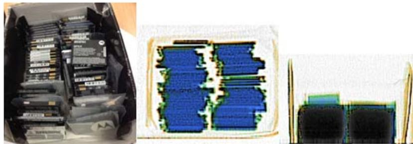
Figure 3. 632DV scans of cell phone batteries. Left: photograph. Middle: X-ray image (vertical view). Right: X-ray image (horizontal view)
