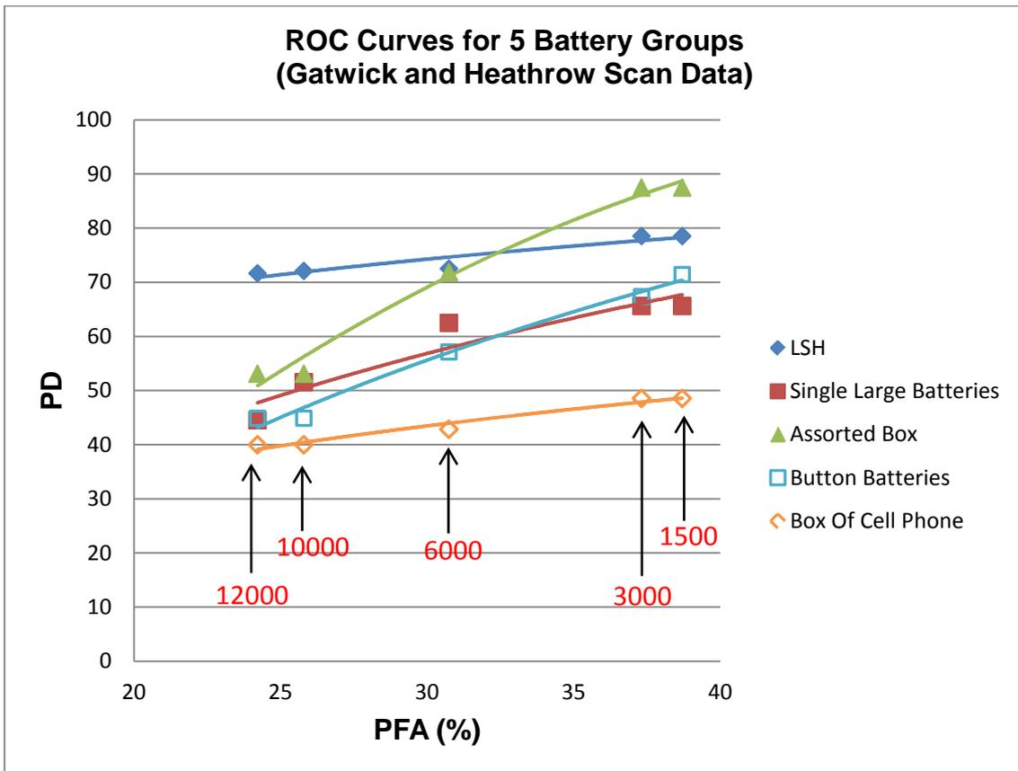
Figure 10. ROC analysis for the five battery groups. The threshold, the minimum area for identifying a region as a Li battery, is varied. The numbers in red indicate the magnitudes (in pixels) of the areas.
