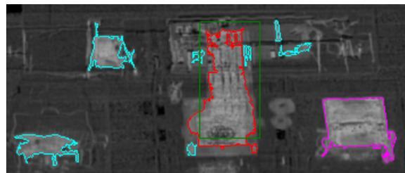
50 cycles Li-ion battery attached to cargo
