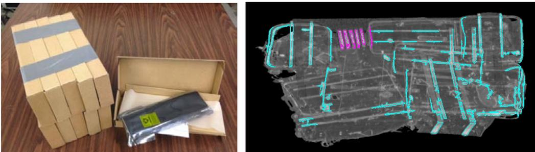
Figure 12. Detection of laptop-computer batteries arranged in 2 rows of 5 batteries. The photograph at the left shows the bulk packaging of the batteries. The image at the right shows the algorithm result. The group of batteries are outlined in purple; the thin purple line at the right of the group is a false alarm. The blue outlines are regions that have been discarded by the algorithm.
