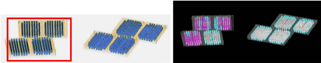
Figure 14. Sample x-ray image (at left) from the Hong Kong data and algorithm detection result (at right). Some structures (within the hand-drawn red box at left) could be Li batteries. Some of these structures yield alarms (regions on the right outlined in purple).
