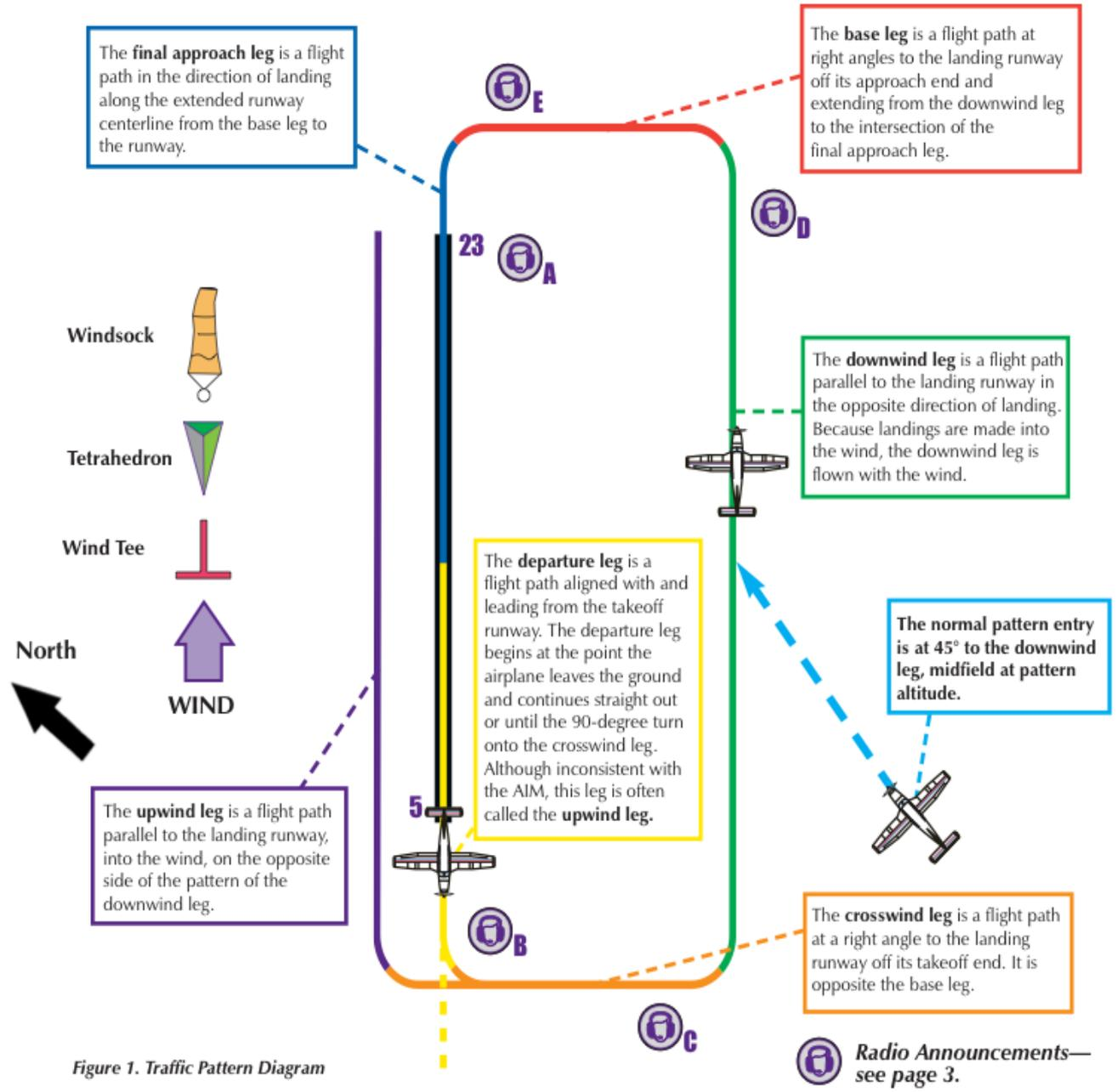
Figure 1. Traffic Pattern Diagram
